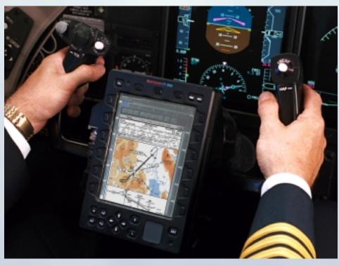
The "lowest" of the three classes might be considered Class 1 since it covers electronic equipment that is completely portable. The next higher class, which allows more capability, is Class 2. It covers PEDs that are mounted to the aircraft in a docking station or cradle that has received a supplemental type certificate (STC). The highest class, with the most capability, is Class 3. It covers EFBs that are installed avionics systems that may have *all* EFB functions.
