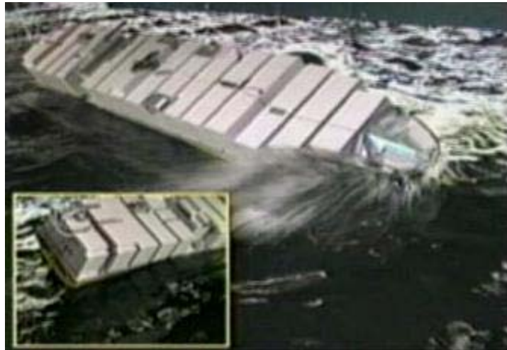
Model test of C11 Class (APL China) experiencing parametric roll in long crested head seas
